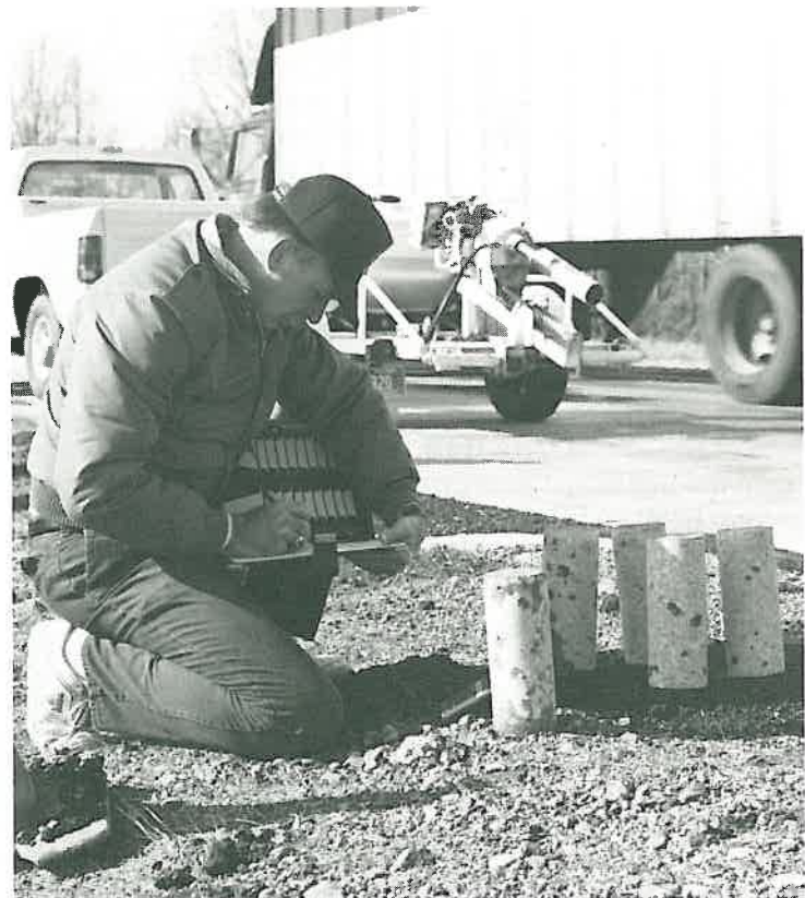
Bill Stagge, Pavement Management Engineer, records information regarding core samples taken from the Forrest City-Interstate 40 test site.
